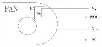
SIGNAL VOLTAGE RANGE:  $0 \sim (V_+ - 0.5) \text{ VDC}$
