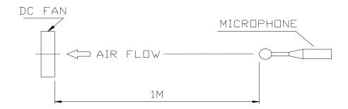
NOISE IS MEASURED AT RATED VOLTAGE IN FREE AIR IN SEMI-ANECHOIC CHAMBER WITH MICROPHONE AT A DISTANCE OF ONE METER FROM THE FAN INTAKE.
